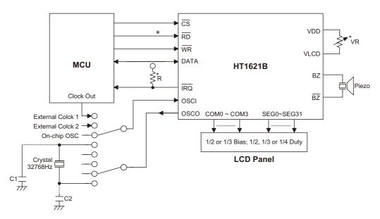
Note: The connection of  $\overline{\text{IRQ}}$  and  $\overline{\text{RD}}$  pin can be selected depending on the requirement of the MCU.
