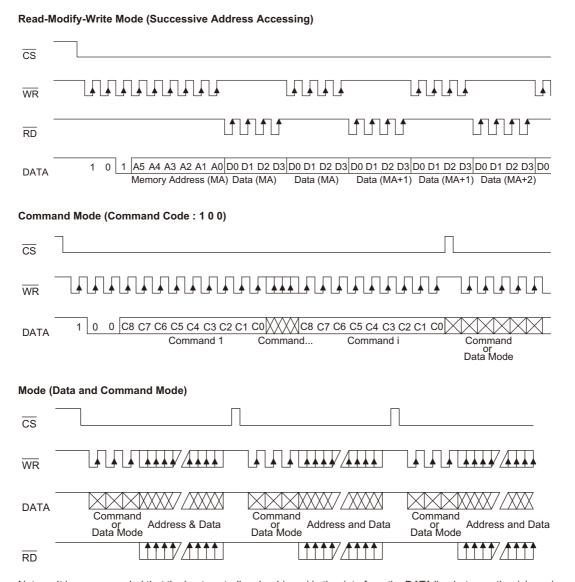
Note: It is recommended that the host controller should read in the data from the DATA line between the rising edge of the  $\overline{\text{RD}}$  line and the falling edge of the next  $\overline{\text{RD}}$  line.
