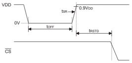
Figure 4 Power-on Reset Timing
